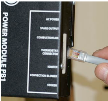
Plug Cable into RJ45 Jack on Power Module
