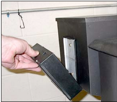
Attaching Power Module to Bracket on side of coal hopper.
