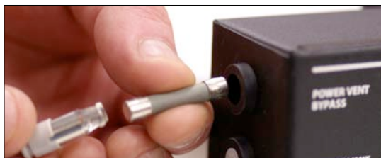
Installing Power Vent Bypass fuse. (10A Slo-Blow)
