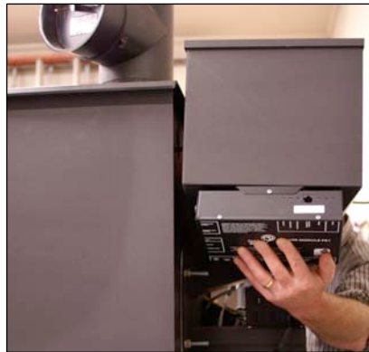
When mounting on bottom of coal hopper, use silicone sealant on bracket mounting screws.
